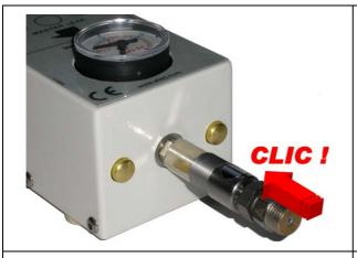
Install the calibrated leak on the output connector of the **CDH6000**.
